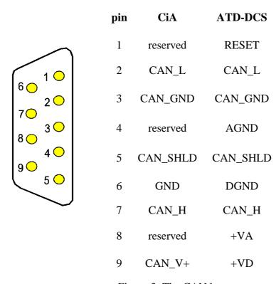
Figure 3 The CAN bus connector
