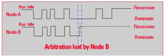
Figure 2 - CAN Bus Arbitration (non-destructive Bitwise Arbitration)
