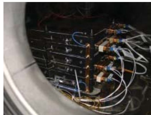
Vacuum test of Smart-1 system unit.
