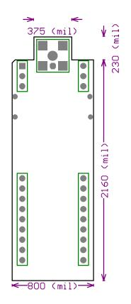
Package fits in 40 PIN DIP socket with 600 mil spacing.
