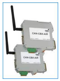
From the In-Rail-Bus individual modules can be removed without interrupting the bus signals.
