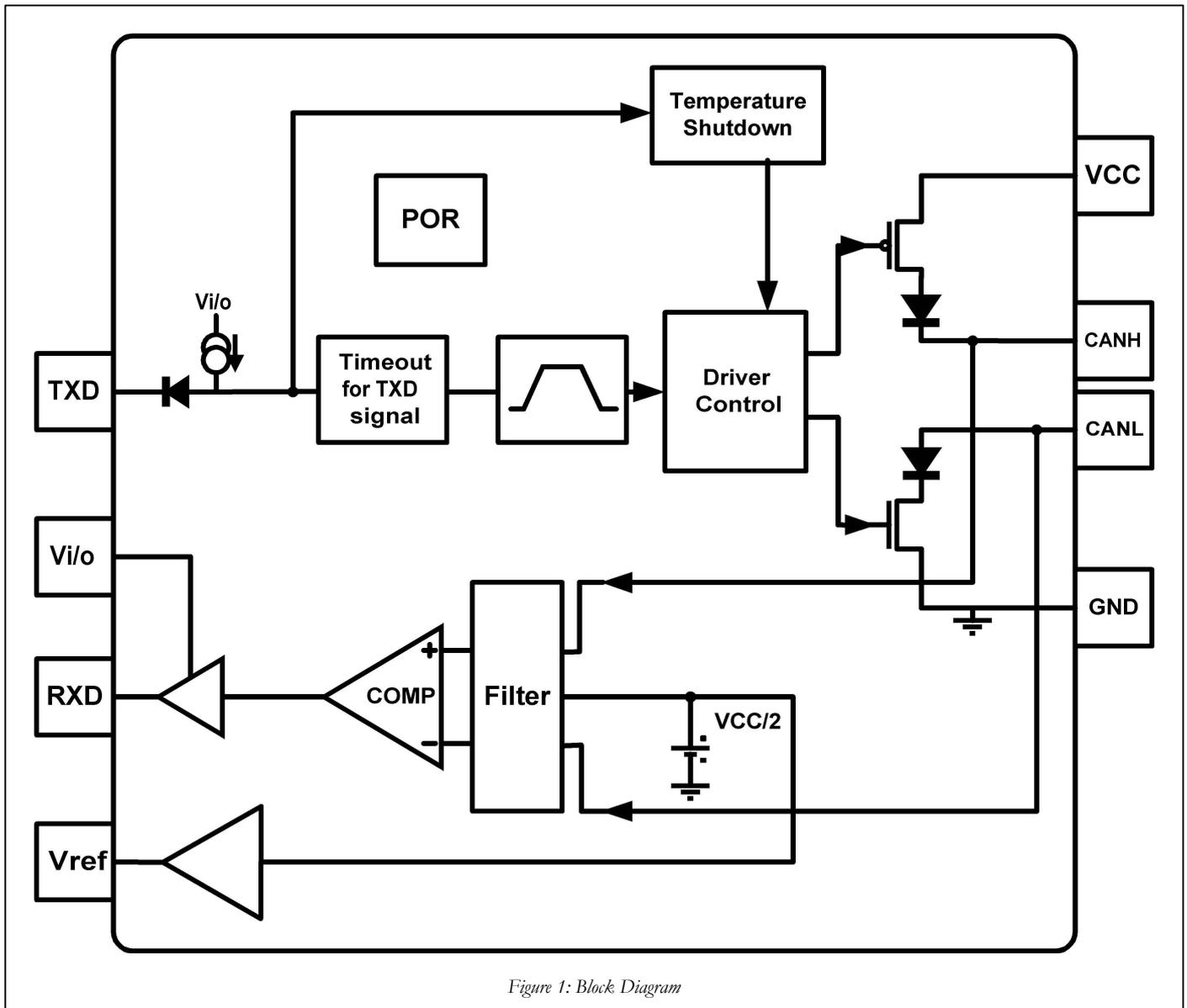
Figure 1: Block Diagram
